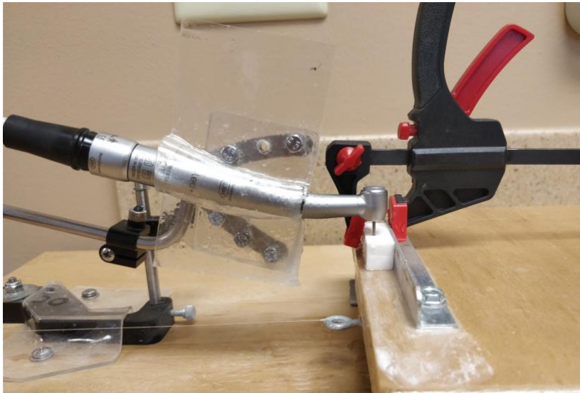
Figure 8. The zirconia specimen mounted on the platform
