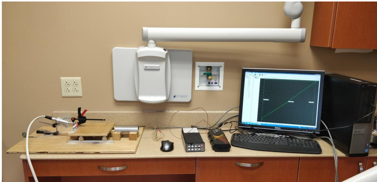
Figure 6 The setup of the experiment. From left to right, apparatus, LVDT signal, personal Daq/3000 and the computer running Daq/3000 software.
